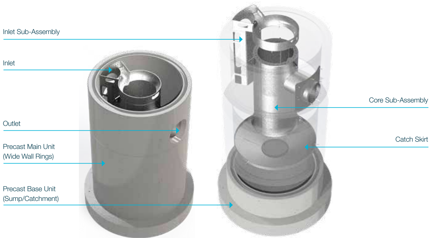
Figure 1 - StormCleanser™ Assembly and Exploded View
